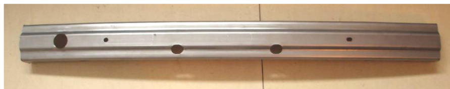
Bumper, HC700/980DP (thickness: 1.6mm)
