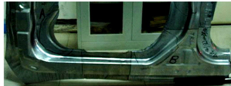
Side panel reinforcement, TWB HC420/780 (Thickness: 1.6mm)
