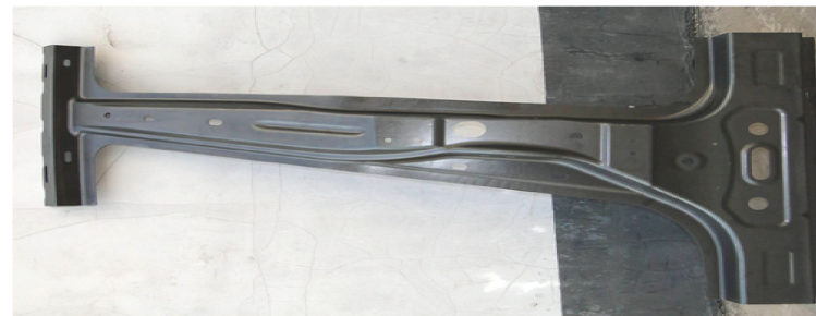
B-pillar B1500HS (Thickness: 1.8mm)
