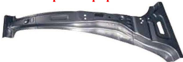
B-pillar reinforcement, HC420/780 (Thickness: 1.8mm)
