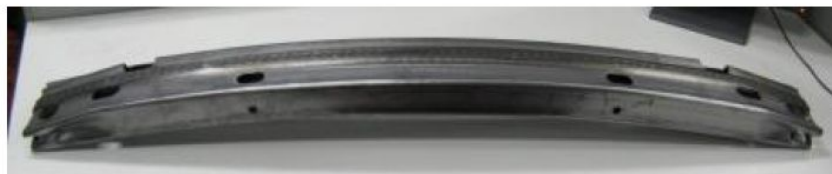
Rear bumper, HC700/980MS (thickness: 1.6mm)
