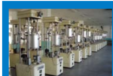
单头持久蠕变试验机 Single-sample Long-time Creep Test Machine
