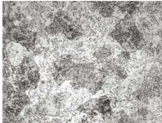
宝钢Cr9Mo的金相组织 ×400 Cr9Mo Metallographic structure of Baosteel ×400
