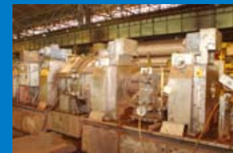
超声波涡流联合探伤机组 Ultrasonic Flaw Detection & Eddy Current Detection Units
