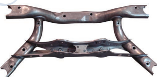
Rear Subframe Cross Beam QStE340TM, 2.7mm
