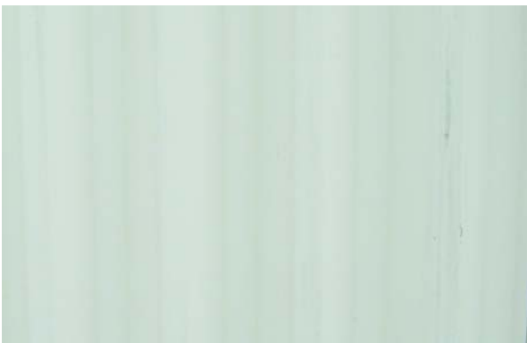
Figure 1: One year after the prepainted steel sheet is applied to the lime wall finish
