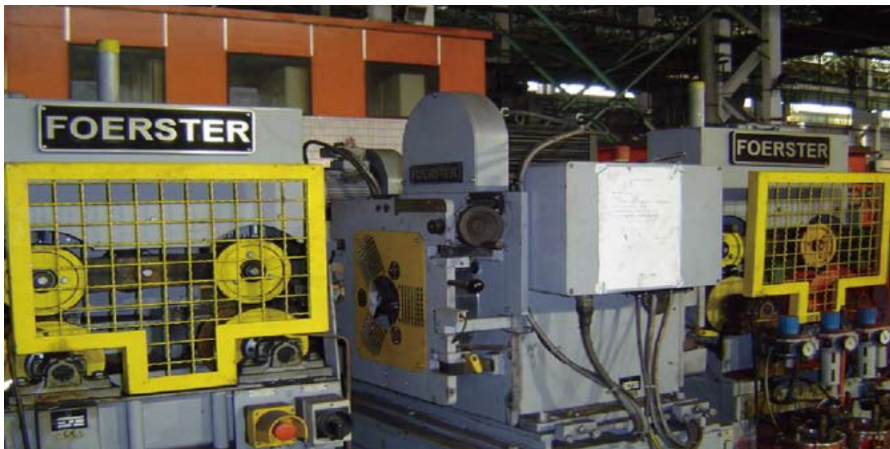
A、B、C、D线棒材漏磁探伤设备 A, B, C, D wire and bar Magnetic flux leakage testing equipment
