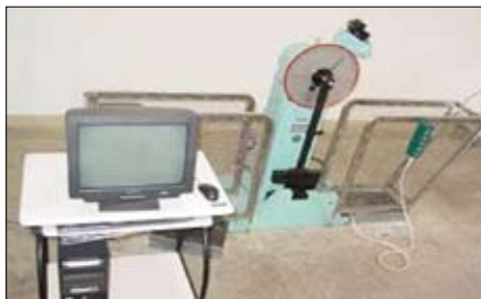
微机控制摆锤式冲击试验机 Pendulum impact testing machine with micro computer control
