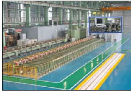
联合探伤机组 Unite fault detection unit
