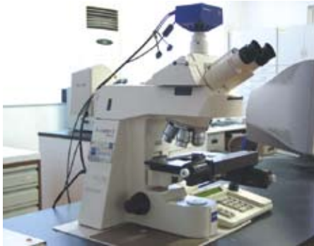
Axioplan-2 正置式金相显微镜 Axioplan-2 metallographic microscope for specimens upward-mounted
