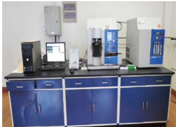
EMGA-620W氧氮联测仪 EMGA-620W oxygen and nitrogen analyzer
