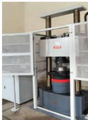
YAW6106液压压力试验机 YAW6106 hydraulic pressure tester
