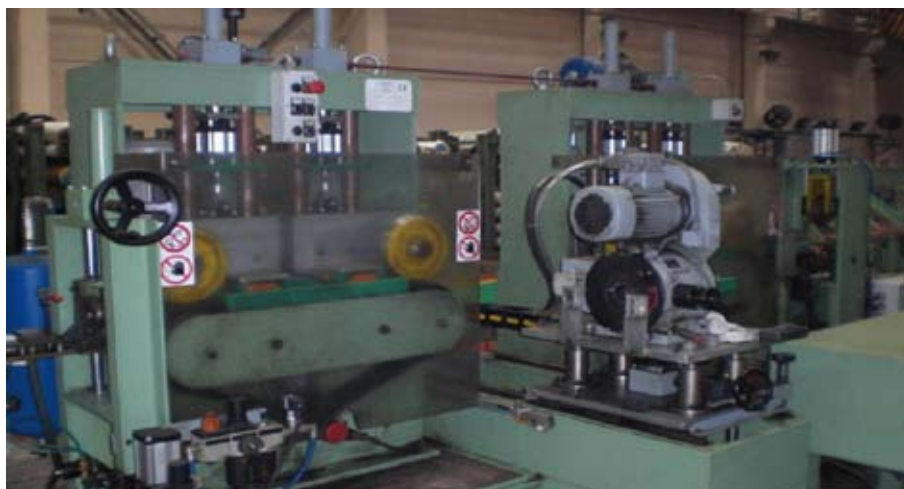
棒材涡流探伤设备 eddy current flaw detection equipment for bars
