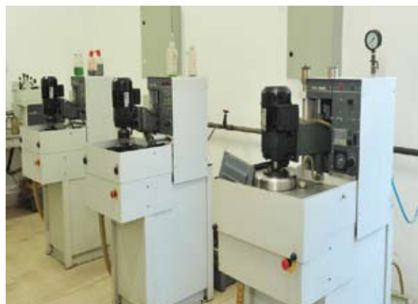
STRUERS 自动磨样设备 STRUERS automatic specimen grinding machine
