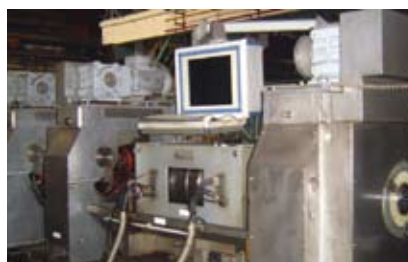
银亮棒材超声探伤设备 ultrasonic flaw detection equipment for bright bars
