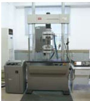
MTS 810电液伺服低周疲劳试验 MTS 810 electrohydraulic servo low-cycle fatigue tester
