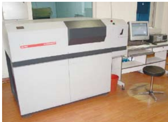
ARL4460光电直读光谱仪 ARL4460 photoelectric direct-reading spectrometer
