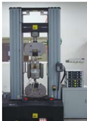
Z150电子式高温拉伸试验机 Z150 electronic elevated temperature tensile tester
