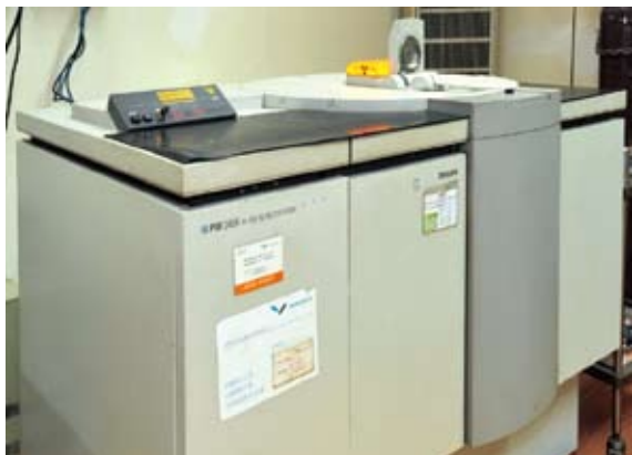
PW2404 X射线荧光分析仪 PW2404 X-ray fluorescence spectrometer
