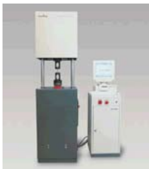
HFP150高频疲劳试验机 HFP150 high-frequency fatigue tester
