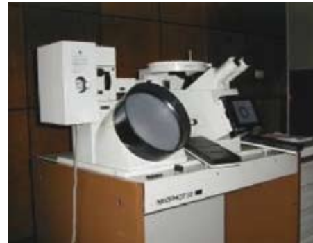
NEOPHOT32 卧式金相显微镜 NEOPHOT32 horizontal metallographic microscope
