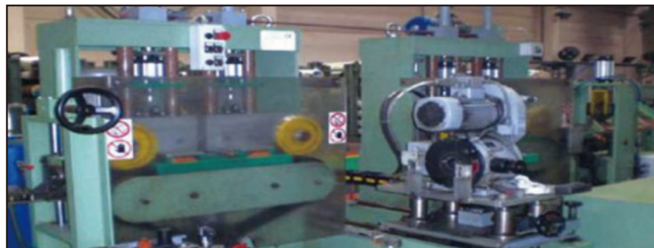
棒材涡流探伤设备 eddy current flaw detection equipment for bars
