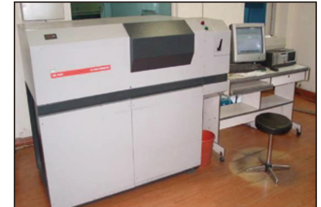
ARL4460光电直读光谱仪 ARL4460 photoelectric direct-reading spectrometer
