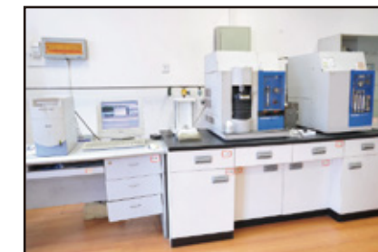
EMGA-621W氢分析仪 EMGA-621W hydrogen analyzer
