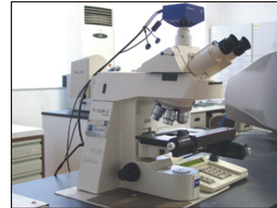
Axioplan-2正置式金相显微镜 Axioplan-2 metallographic microscope for specimens upward-mounted
