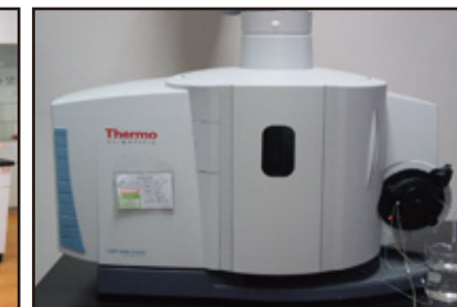
电感耦合等离子体发射光谱仪 inductively coupled plasma emission spectrometer
