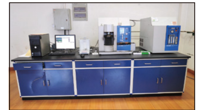
EMGA-620W氧氮联测仪 EMGA-620W oxygen and nitrogen analyzer
