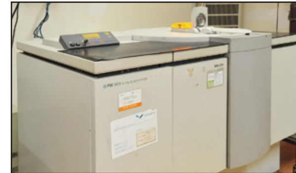
PW2404 X射线荧光光谱仪 PW2404 X-ray fluorescence spectrometer
