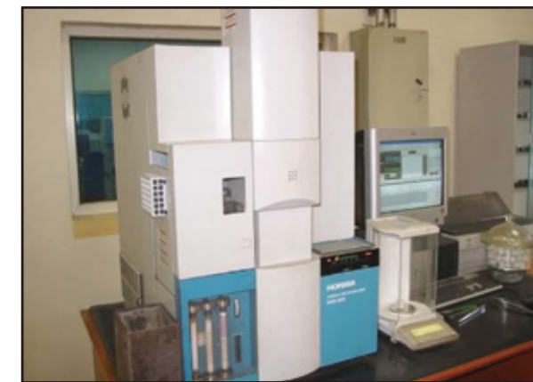
EMIA-820V红外碳硫分析仪 EMIA-820V infrared carbon and sulfur analyzer
