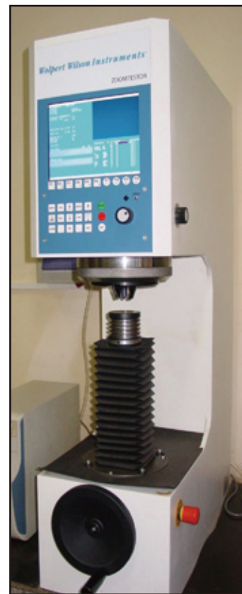
ZOOMTESTOR布、洛、维三用硬度计 ZOOMTESTOR Brinell, Rockwell, Vickers hardness tester
