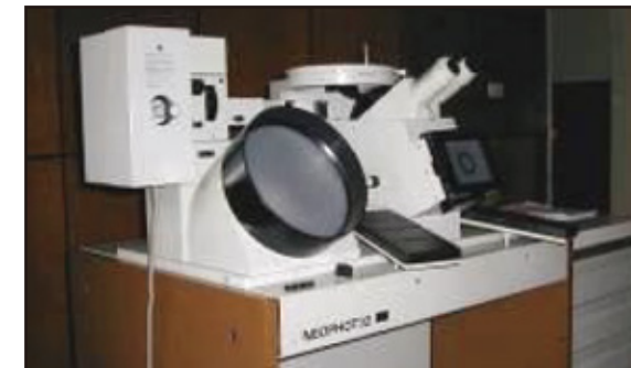
NEOPHOT32卧式金相显微镜 NEOPHOT32 horizontal metallographic microscope
