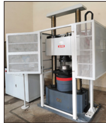
YAW6106液压压力试验机 YAW6106 hydraulic pressure testing machine
