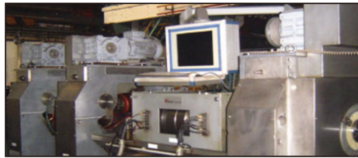
银亮棒材超声探伤设备 ultrasonic flaw detection equipment for bright bars
