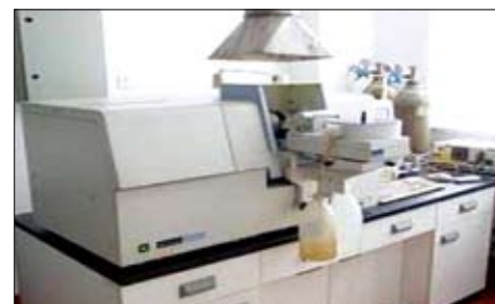
AA600石墨炉原子吸收光谱仪 AA600 Graphite Furnace Atomic Absorption Spectrophotometer
