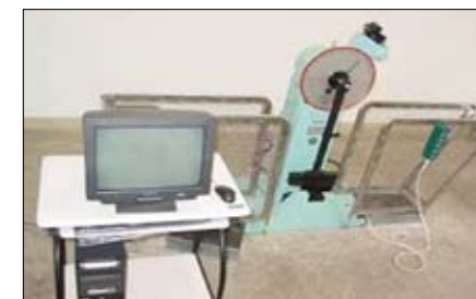
微机控制摆锤式冲击试验机 Pendulum impact testing machine with micro computer control
