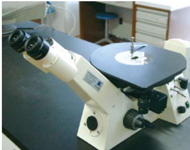
AXIOVERT25CA金相显微镜 AXIOVERT25CA metallographic microscope
