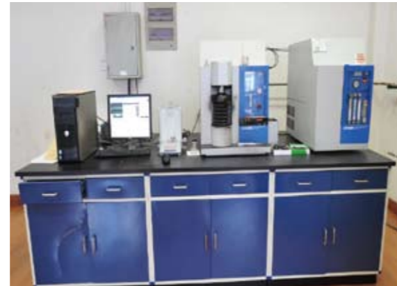
EMGA-620W氧氮联测仪 EMGA-620W oxygen and nitrogen analyzer
