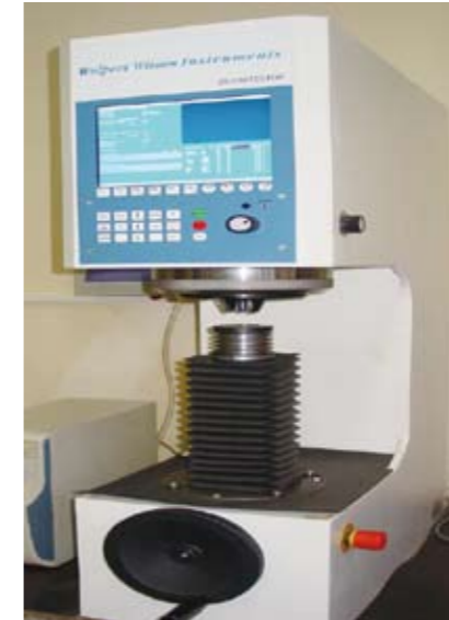
ZOOMTESTOR布、洛、维三用硬度计 ZOOMTESTOR Brinell, Rockwell, Vickers hardness tester
