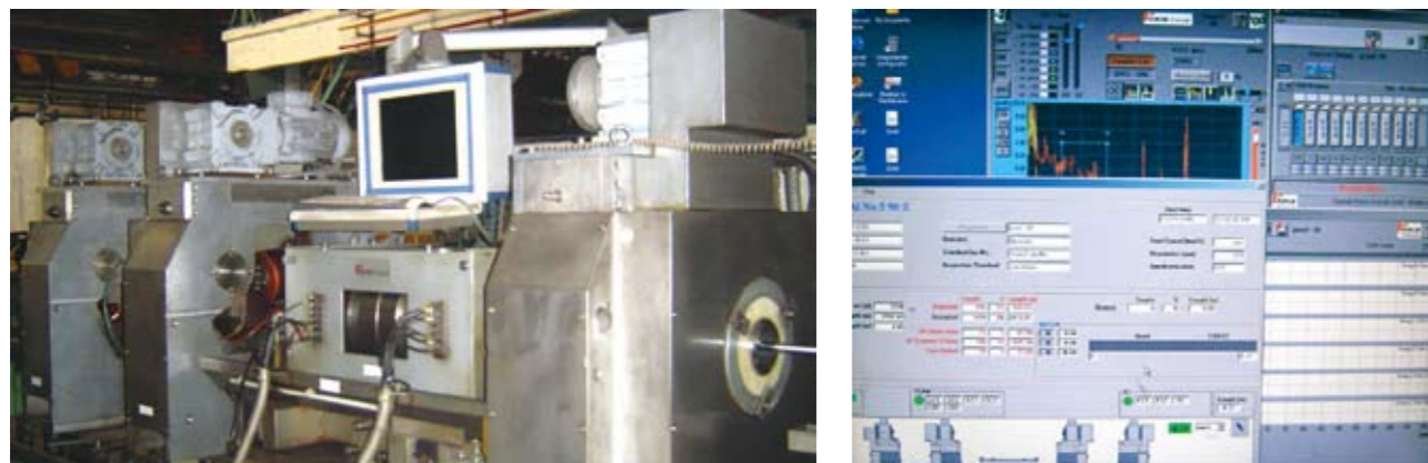
银亮棒材超声探伤设备 ultrasonic flaw detection equipment for bright bars
