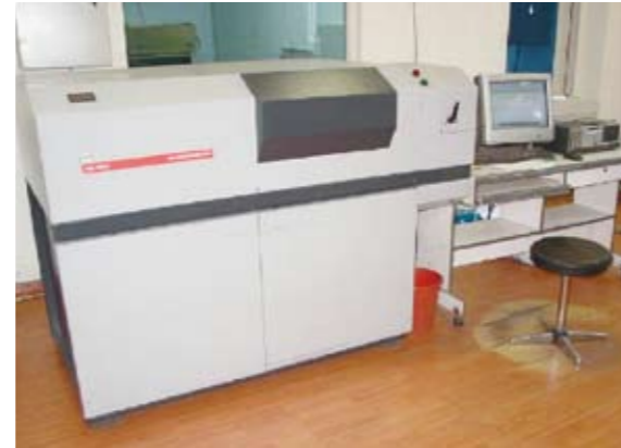
ARL4460光电直读光谱仪 ARL4460 photoelectric direct-reading spectrometer
