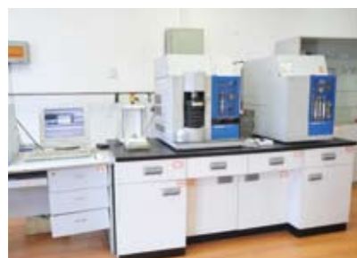
EMGA-621W氢分析仪 EMGA-621W hydrogen analyzer
