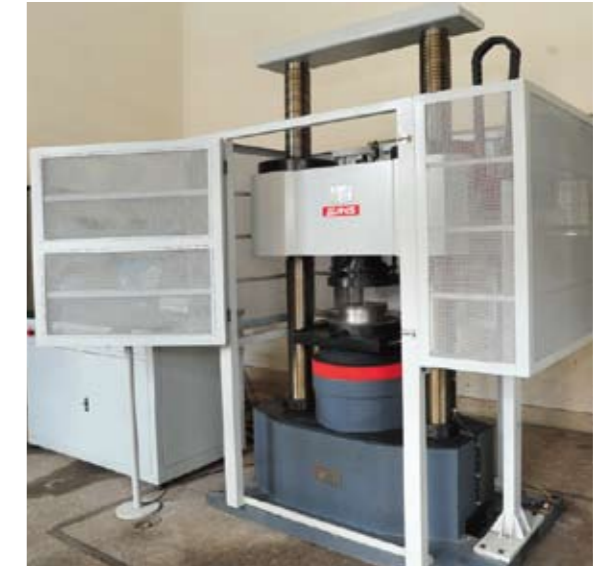
YAW6106液压压力试验机 YAW6106 hydraulic pressure testing machine
