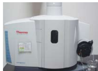
电感耦合等离子体发射光谱仪 inductively coupled plasma emission spectrometer
