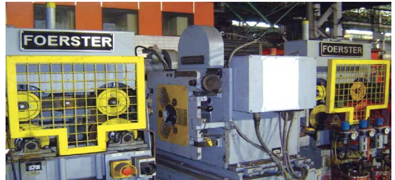
A、B、C、D线棒材漏磁探伤设备 magnetic flux leakage testing equipment for wire and bar installed in Line A, Line B, Line C and Line D
