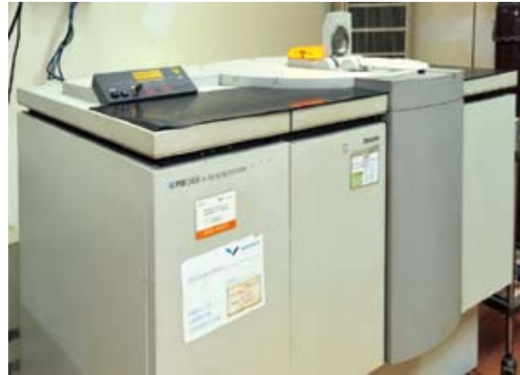
PW2404 X射线荧光光谱仪 PW2404 X-ray fluorescence spectrometer
